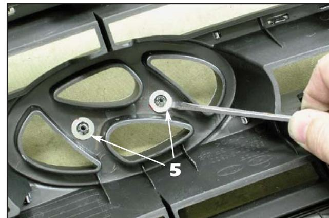
5. Remove the factory emblem from the grille by removing the push on retainers securing the emblem into the factory emblem recess. Insert a small flat blade screwdriver in between the retainer and the grille and twist to remove.
