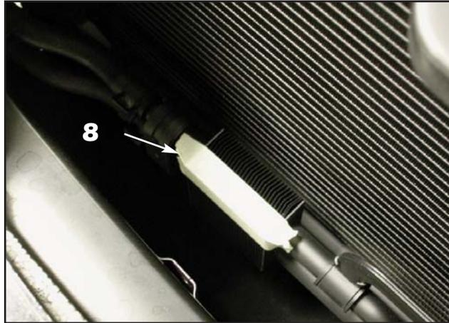
8. **IMPORTANT:** Use masking tape to cover the fins on the small cooler located on the passenger side near the bottom of the radiator. **The fins are very sharp and you could easily cut yourself while installing the mounting hardware on the lower mesh grille.**
