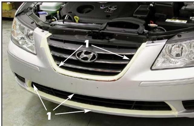
1. Open the hood and carefully apply several layers of masking tape to the painted upper and lower grille openings (around the upper factory grille). This will protect the painted surfaces during grille installation.
