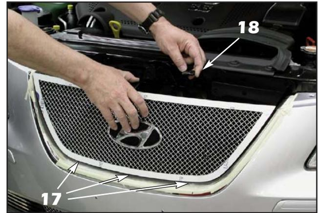
17. Align the mounting pins on the bottom of the Mesh grille into the slots made in Step 16.
