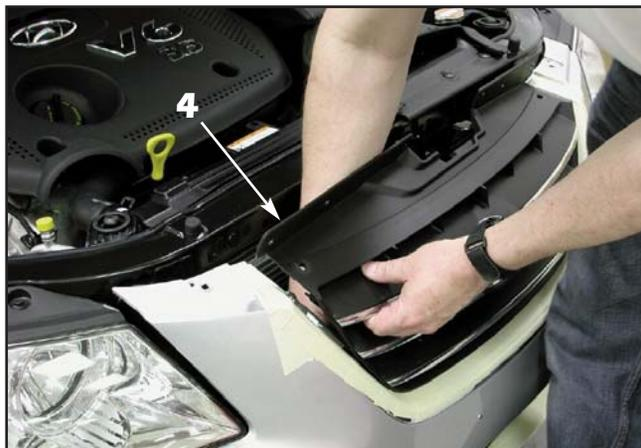
4. Remove the factory upper grille from the bumper cover by removing the phillips screws located at the sides and bottom of the grille. A short phillips screwdriver or ratcheting screw driver works best.
