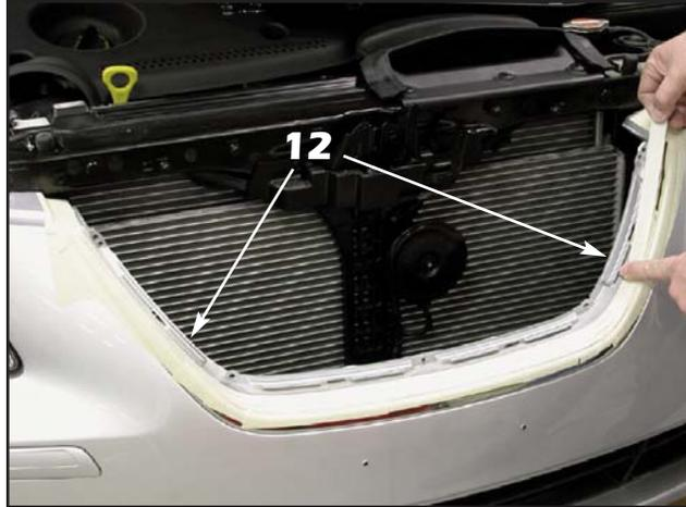
12. Apply additional masking tape 1/4" inside the line taped in **Step 1** around the upper grille opening.
