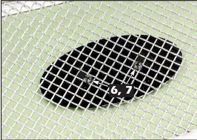
6. Align the factory emblem removed in **Step 5** onto the emblem mounting plate and through the partial holes lasered in the mesh section. The factory emblem studs will push through the partial holes in the mesh for a tight fit.
