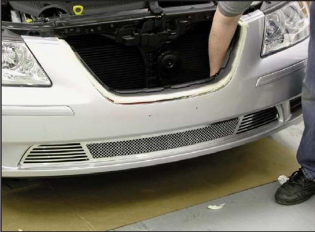
11. Install the lower grille section first, accessing the mounting hardware from the top. The rectangular 3 hole mounting brackets install over the studs and the black plastic washers install on the remaining studs. Snug the hardware but do not overtighten as you will indent the lower grille frame where the studs are located.
