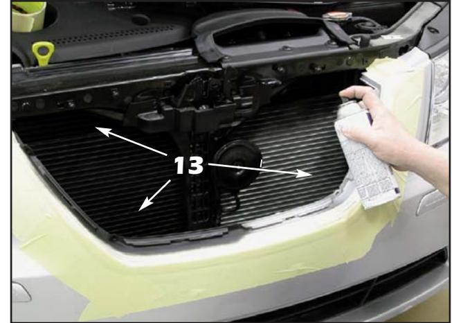
13. Apply flat or semigloss black paint to everything that will be visible through the E&G grille once it is installed. On vehicles painted colors other than dark blue or black, use a scotch brite pad to scuff the paint around the grille opening and paint the return edge of the grille opening inside the mounting pin holes as well.
