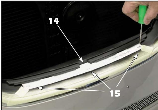
14. Cut out and align the supplied hole location template onto the bumper cover, making sure that the center notch in the template line up with the center recessed area in the bumper cover.
