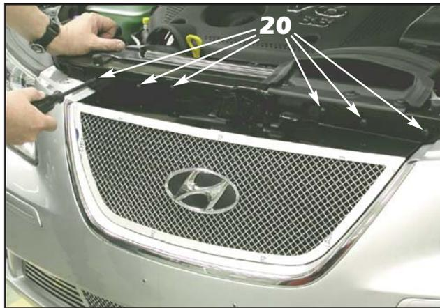
20. Make sure that the E&G mesh grille is centered and level, then reinstall the factory upper screws to secure the E&G grille top plate to the core support (press down on the grille when tightening the screw but **DO NOT OVER TIGHTEN!** You could strip out the screw holes.
